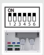
Set the inverter dial code (INV SET) to all up (111111) as shown above before proceeding with Wi-Fi setup.
