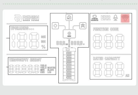
After completing the steps, the WiFi icon on the battery screen will blink, indicating it's connected to the router. Then, set the inverter code to "000000".
